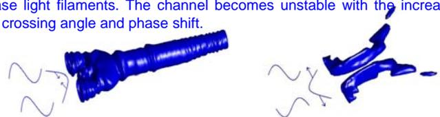
The energy fluence distribution of two merging (left) and repulsing (right) light filaments.
